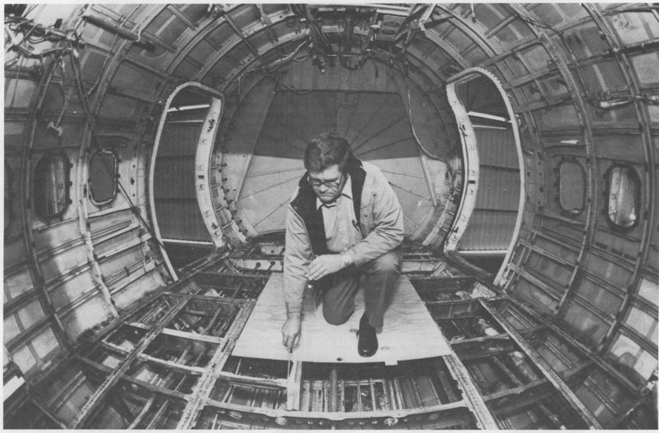
HOLLOW SHELL — Ken Harmon of Aerodynamics Dept. 1554 examines the interior of a 737 transport plane to be used as part of Aging Aircraft Non-destructive Inspection Validation Center research at Sandia. (Photos by Randy Montoya)
